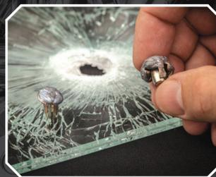
To ensure they perform when the stakes are high, duty rifle loads go through the grueling FBI protocol. This series of tests evaluate ballistic performance benchmarks including a bullet's penetration, expansion and weight retention after passing through common barriers like clothing, wallboard and auto glass. The higher the score, the more equipped a given round is to stop the threat and minimize collateral risks. Federal and Speer duty rifle loads are some of the highest-scoring available.
